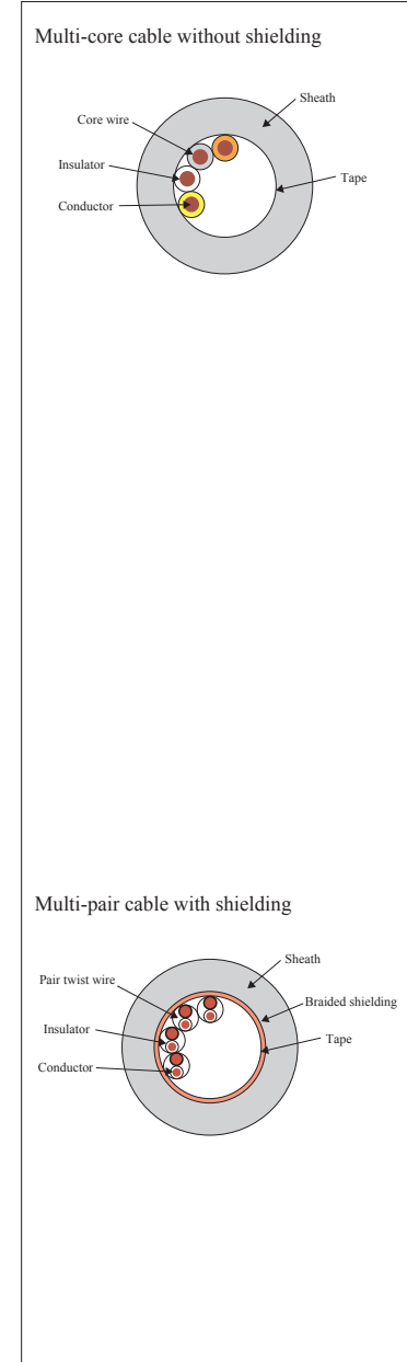
(Table 2) Configuration of multi-pair cable with shielding
